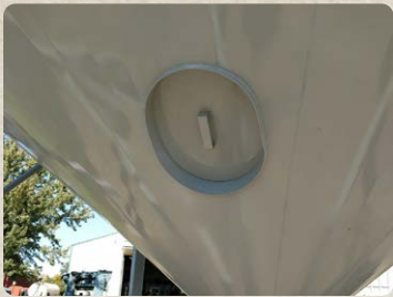
Manhole with Cover
